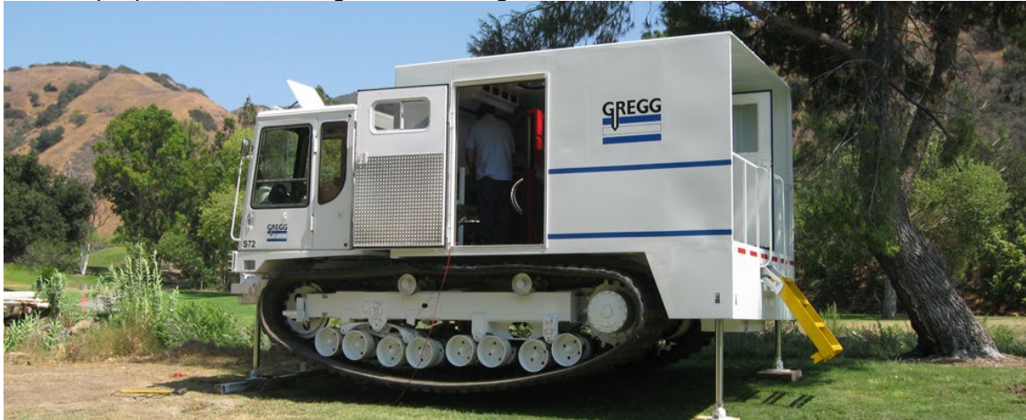
Figure 1: Cone Penetrometer Test (CPT) Rig Example Photo
